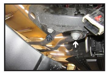
5. **Trucks with Tow Hooks:** Using a 21MM socket remove the front bolt (gray), and then using an 18MM socket remove the back bolt (white) attaching the tow hook to the frame. Remove tow hook. Do this on both sides of the vehicle. The tow hooks will not be reinstalled.
