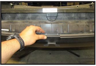
17. Hold electrical bracket on top of the bumper/fascia and mark holes. Using a 7/32" drill bit, drill two (2) holes.Note: Recommend spraying holes with an anti-rust spray to prevent future rust.
