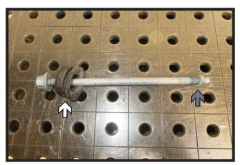
6. **Trucks with Tow Hooks:** Remove rubber grommet (white) and metal piece (gray) from back tow hook bolt. Reinstall the tow hook bolt and hardware. Do this on both sides of the vehicle.
