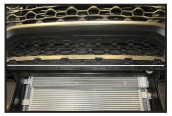
11. Using a reciprocating saw, cut a straight line (white line) across the plastic piece to remove the indicated area.
