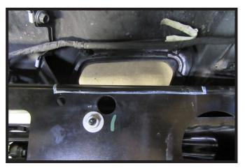
Using a reciprocating saw trim the indicated area above the tow hook opening from the metal piece on the back of the bumper as shown. Do this on both sides of the vehicle.
