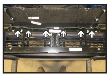
8. Remove the six (6) clips attaching the wire loom to the bottom of the shutter housing on the back of the bumper.
