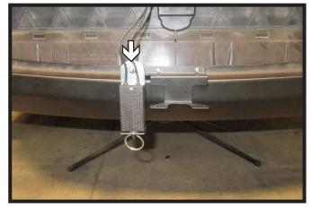
19. **Optional**: Attach breakaway switch to the electrical bracket using the provided hardware.
