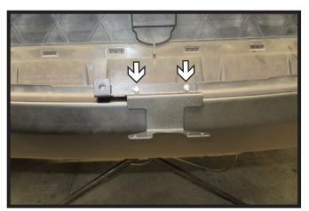
18. Install electrical bracket to the top of the bumper/fascia using the provided hardware.
