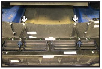
7. Using a T40 Torx remove the two (2) bolts (white) from the bottom of the brackets on the backside of the fascia. Then using a 10MM socket, remove the two (2) bolts (gray) from the top of the brackets. Remove brackets, they will not be reinstalled.
