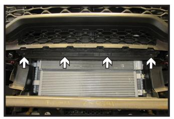
10. Remove the four (4) push pins from rubber piece below grille and remove. It will not be reinstalled.
