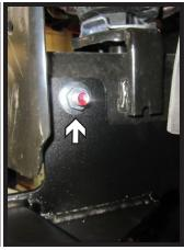
14. Place spacer plate onto 1/2" carriage bolt. Insert bolt and plate through access hole in the front of the vehicle frame. Install bolt and plate into side hole in baseplate and attach 1/2" flange whiz nut. Hand tighten. Do this on both sides of the vehicle.
