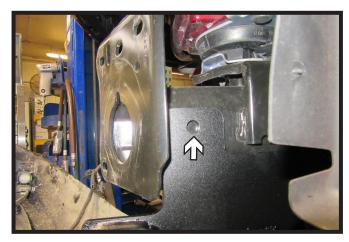
13. Using a 1/2" drill bit, drill the bottom hole and side hole in the frame using the baseplate as a template. Do this on both sides of the vehicle.
