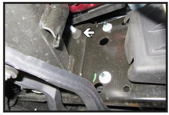
3. Using an 18MM socket, Remove the three (3) nuts from the back side of the bumper. Do this on both sides of the vehicle.
