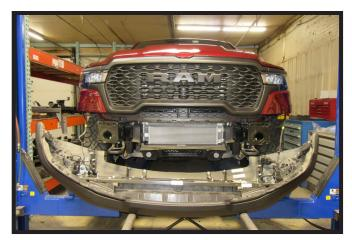
Remove bumper but do not disconnect upper electrical connection on each side.
