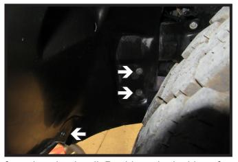
1. Using an 8MM socket, remove the five (5) bolts from the wheel well. Do this on both sides of the vehicle.
