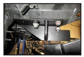
12. Raise baseplate into place and start the 14MM bolt with flat washer and nylon lock nut, hand tighten. Do this on both sides of the vehicle.
