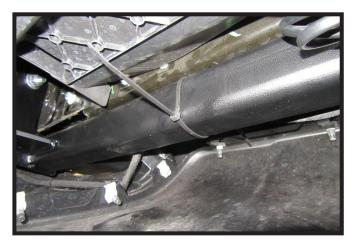
20. Reinstall bumper/fascia. Secure wire loom to the on the back of the fascia to the baseplate using the provided zip ties.
