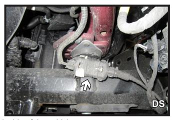
2. Unplug the one (1) electrical connection on each side of the vehicle.
