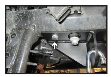
15. Install the 1/2" x 1-1/2" bolt with lock washer and whiz nut into the bottom back hole. Fully tighten all bolts at this time starting with the side bolt, then back bottom bolt, and finally the front bottom bolt. Do this on both sides of the vehicle.
